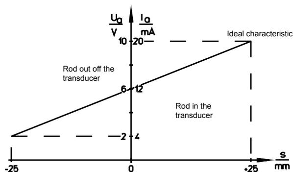
Fig. 17: Current vs. voltage vs. displacement diagram for transducers with electronics A WA F 025 A01 / A02
