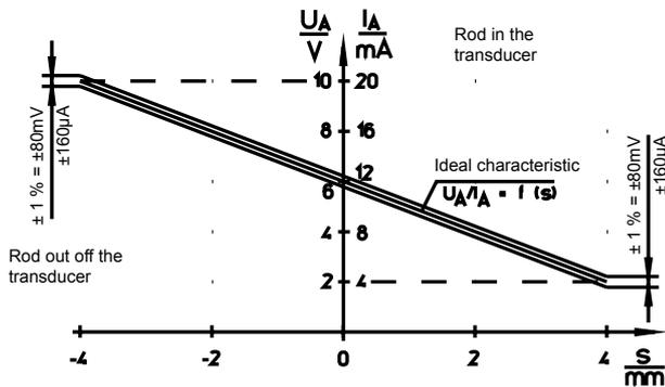
Fig. 6: Current vs. voltage diagram for transducer with electronics A WA X 004 A01
